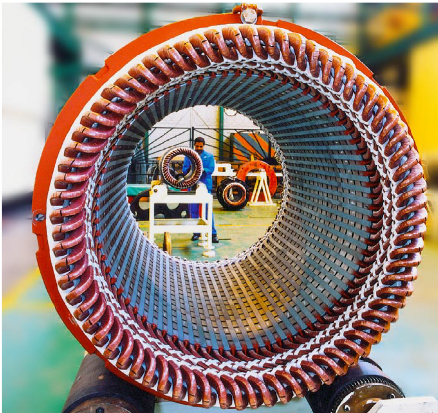
7Mw UNIBOX stator core ready for vacuum impregnation.
