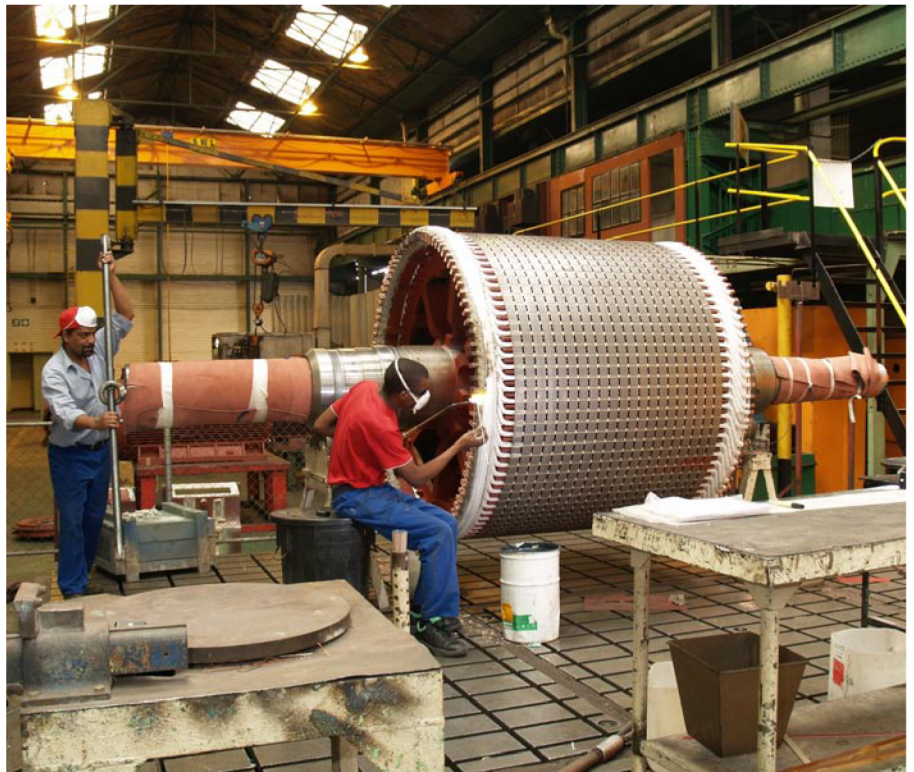
Construction of a standard wound rotor assembly.
